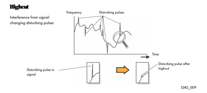
If interference occurs in the upper frequency range due to multipath reception, it will be suppressed by the highcut function in the FM tuner of the car radio.
