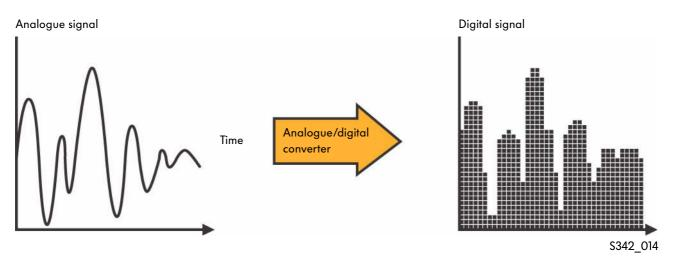
The analogue music signal is converted to a digital signal by an analogue/digital converter.
