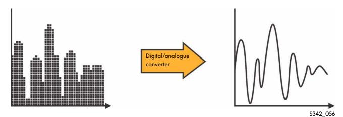
To obtain a suitable signal from the digital signals for playback via the speakers, an analogue signal needs to be formed again in the CD player using a D/A converter.
