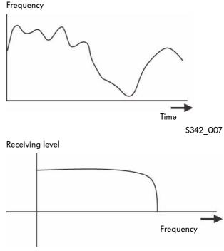
The audio amplifier in the car radio amplifies all frequencies that can be heard by the human ear to a level appropriate to the human sensory range.
