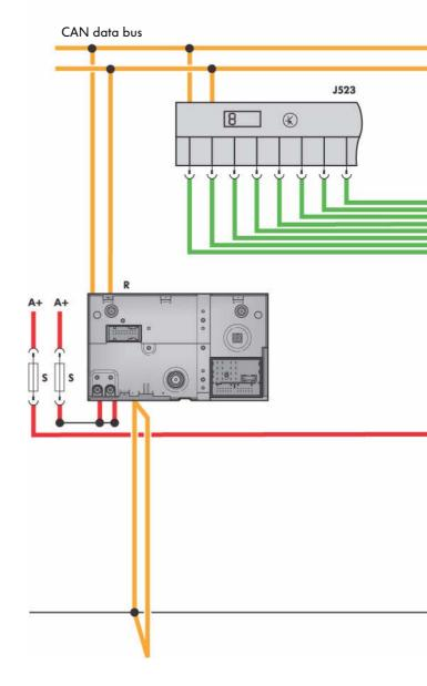
Input signal Output signal Voltage supply (plus) Earth (minus) CAN data bus line
