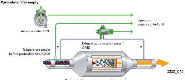
Particulate filter empty = low resistance to flow
