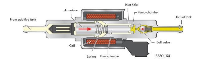
When not energised, the pump is filled with additive. As soon as the engine control unit actuates the particulate filter additive pump, the coil is energised and the armature moves the pump plunger against spring pressure. The pump plunger closes the inlet hole to the pump chamber and forces the additive in the chamber towards the ball valve.
