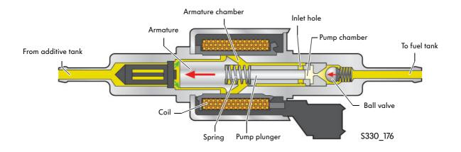
During intake, the additive flows into the armature chamber. The magnetic coil is not actuated by the engine control unit and the spring presses the pump plunger back. At the same time, the ball valve closes the pump chamber.
