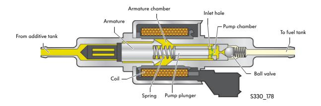
The pump plunger moves to the start position.
