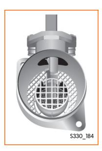
The hot film air mass meter is installed in the intake manifold. Using the air mass meter, the engine control unit can determine the actual mass of intake air.
