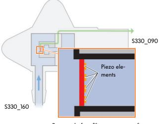
Pressure before filter = pressure after filter
