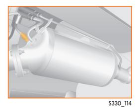
It can be found in the exhaust system before the diesel particulate filter. There it measures the temperature of the exhaust gas.
