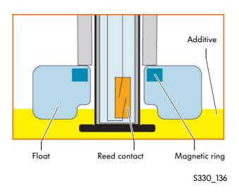
Installed in the shaft of the fuel additive tank sender is a reed contact. It is activated by the magnetic ring installed on the float. If there is sufficient additive in the tank, the float will be in contact with the upper stop. The reed contact is open.
