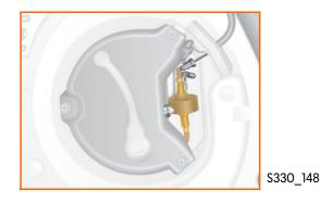
Each time the fuel tank is replenished, the pump is actuated by the engine control unit in a cycle to ensure the correct amount of additive is added.
