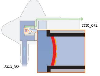
Pressure before filter > pressure after filter
