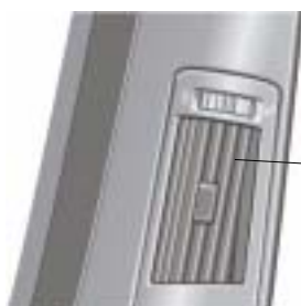
Vents in B-pillar
