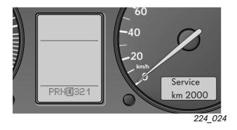
In the standard variant of the dash panel insert, the service information appears in the speedometer counter.
