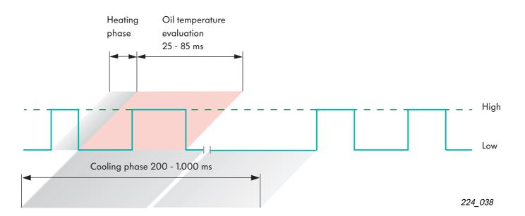
The signal indicates the heating phase as high voltage and the cooling phase as low voltage.
