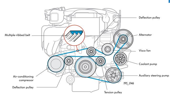
In the longitudinally mounted engine the coolant pump is located on the auxiliary holder. As a result, this engine is slightly shorter than the transversely mounted engine.
