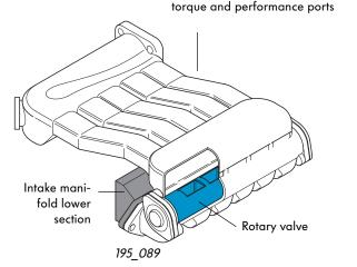
Intake manifold upper section with
