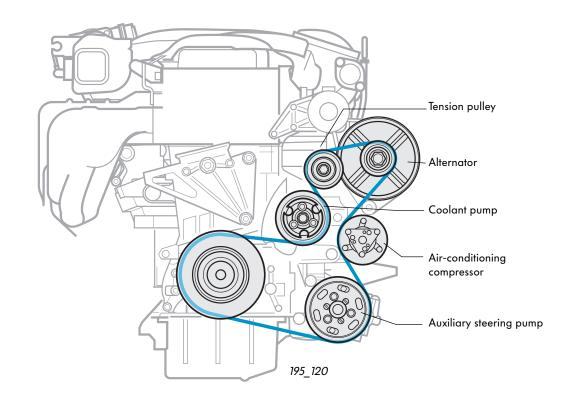
Belt routing in the transversely mounted V5 engine with air-conditioning compressor
