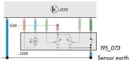
The idling switch utilises the sensor earth of the engine control unit.
